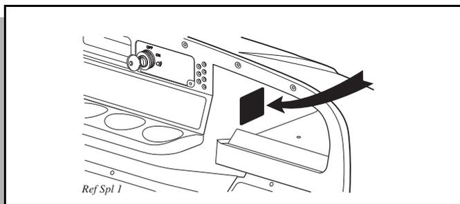
**Fig. 14 Serial Number Plate Location - Early Production**
