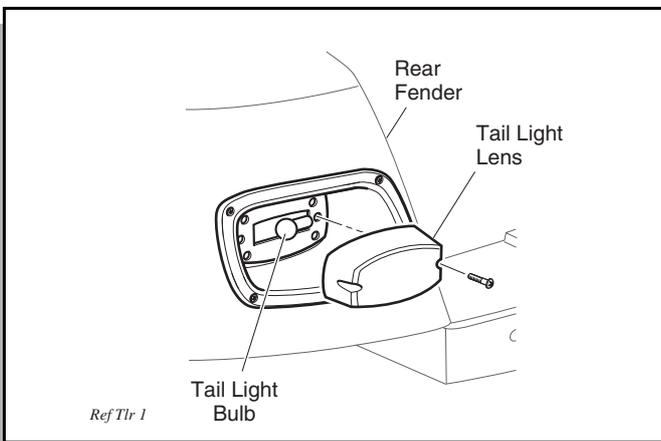
**Fig. 13 Tail and Brake Light Bulb Replacement**
