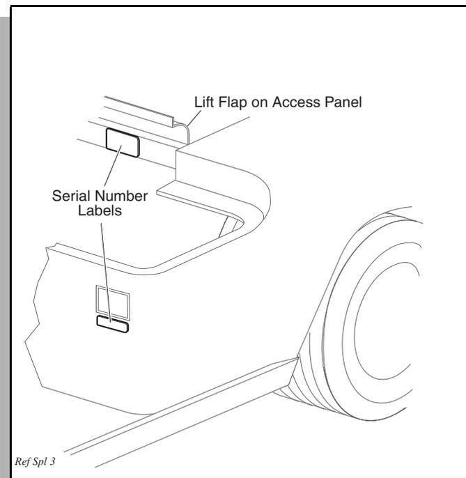
**Fig. 15 Serial Number Plate Location - Late Production**
