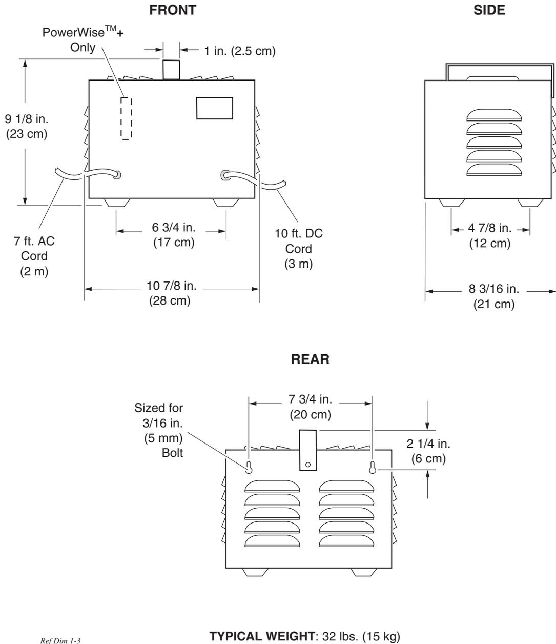
**Fig. 38 PowerWise™ Portable Battery Charger Dimensions**
