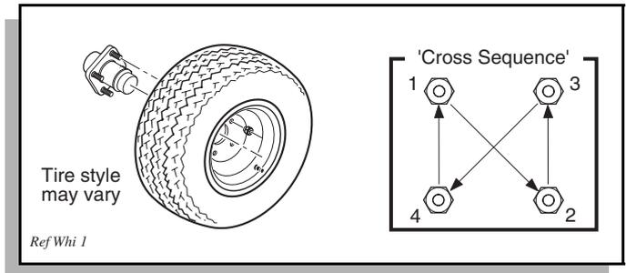
Fig. 11 Wheel Installation
