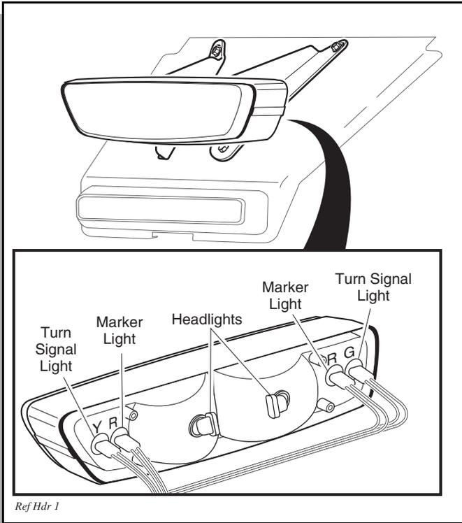
**Fig. 12 Headlight, Turn Signal & Marker Light Bulb Replacement**
