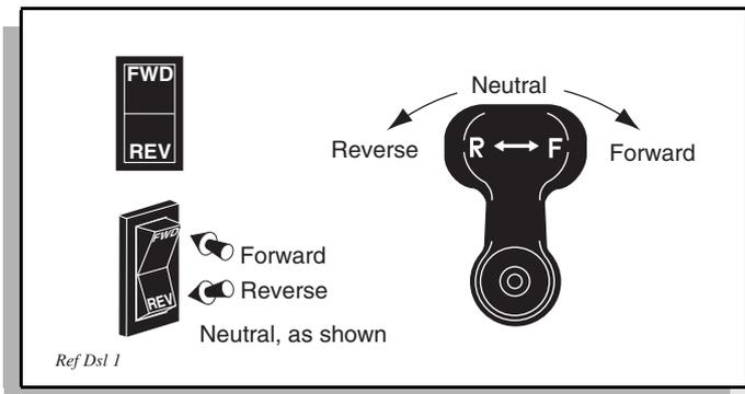
Fig. 5 Direction Selector Types
