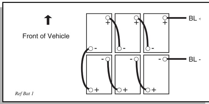
Fig. 28 Battery Connections
