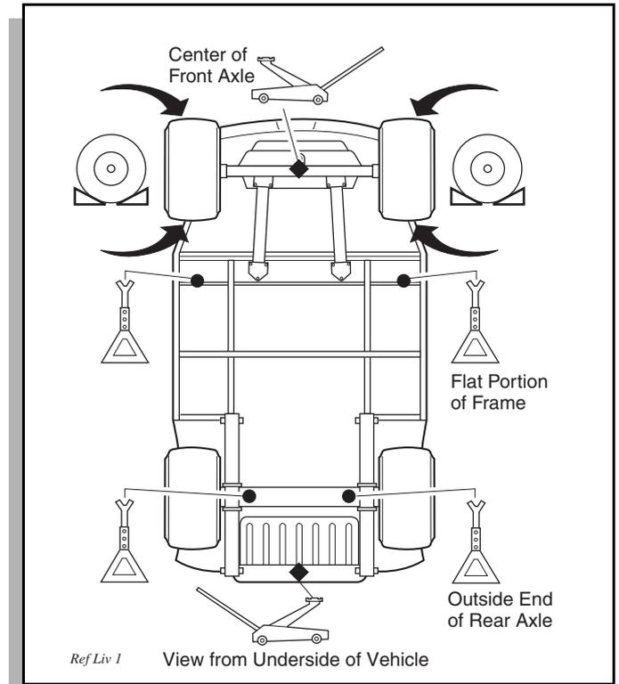
Fig. 10 Lifting the Vehicle
