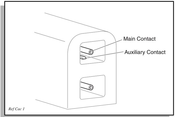
**Fig. 32 Cleaning Auxiliary Contact in Charger Plug**
