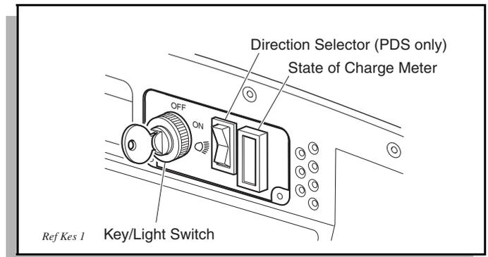
**Fig. 4 Key/Light Switch & State of Charge Meter**
