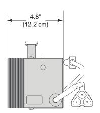
Fig. 3 Battery Charger Dimensions
