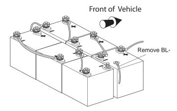
Fig. 1 Disconnect Battery Cable
