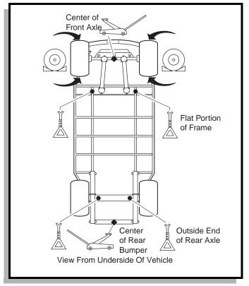
Fig. 2 Lifting the Vehicle
