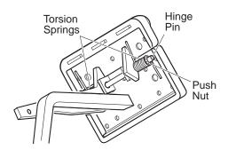
Fig. 11 Parking Brake Pedal Hinge Inspection
