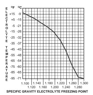
Fig. 6 Freezing Point of Electrolyte Battery Charging
