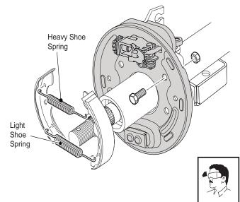
Fig. 17 Orientation of Brake Shoe Springs
