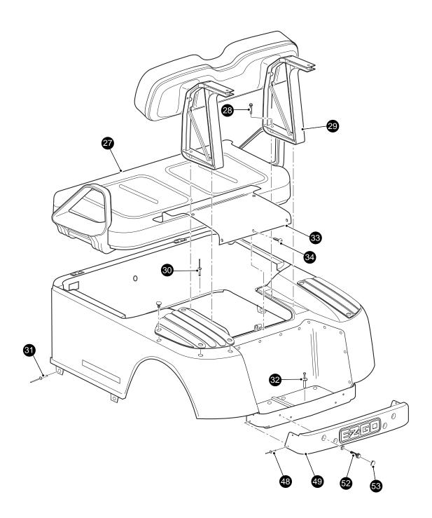
Fig. 3 Body Components (Rear)
