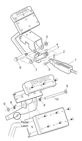
Fig. 28 Brake Pedal Removal and Installation
