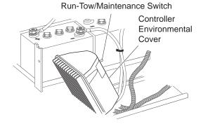
Fig. 1 Run-Tow/Maintenance Switch
