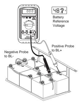
Fig. 4 Battery Reference Voltage
