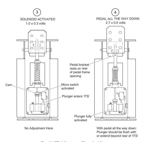
Fig. 12 ITS Adjustment (Sheet 2 of 2)
