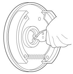
Fig. 5 Removing/Installing Inner Snap Ring
