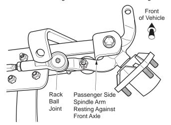
Fig. 18 Spindle Contact with Front Axle
