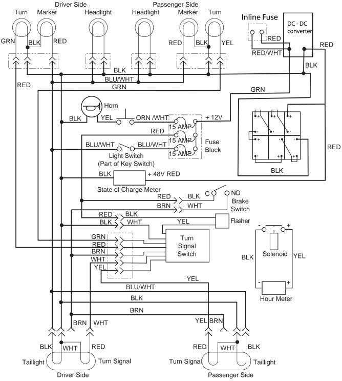
For vehicles without turn signals, remove WHT wire from left rear turn signal remove YEL wire from right rear turn signal connect BRN wire to RED
