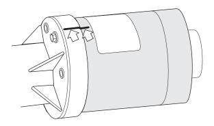
Fig. 2 Mark Axle and Motor
