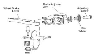
Fig. 15 Adjuster Mechanism
