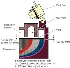
Fig. 1 Correct Electrolyte Level
