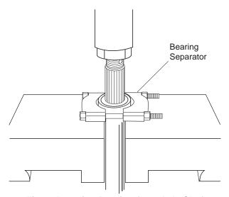
Fig. 4 Pressing Bearing from Axle Shaft
