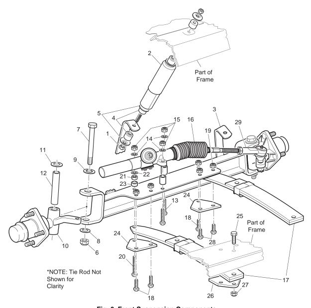
Fig. 6 Front Suspension Components
