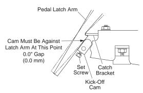
Fig. 12 Kick-Off Cam Inspection
