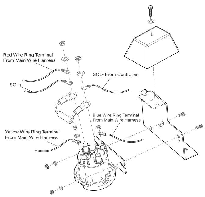
Fig. 13 Solenoid Wiring
