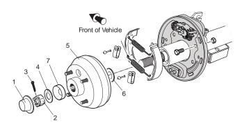
Fig. 21 Brake Assembly
