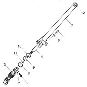
Fig. 22 Steering Shaft and Column
