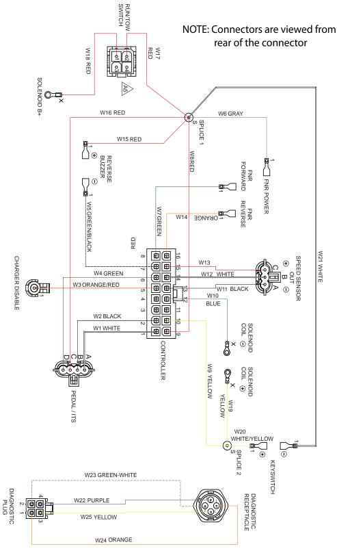
Fig. 3 Main Harness Wiring Diagram
