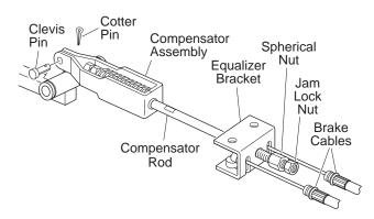
Fig. 26 Brake Cable, Equaliser and Compensator
