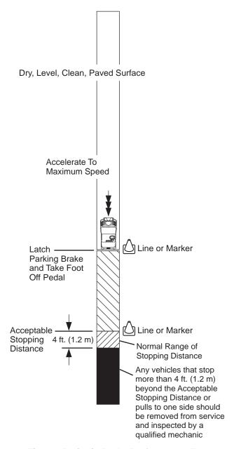
Fig. 13 Periodic Brake Performance Test
