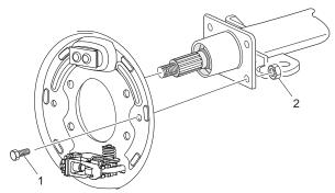
Fig. 23 Backing Plate Removal and Installation
