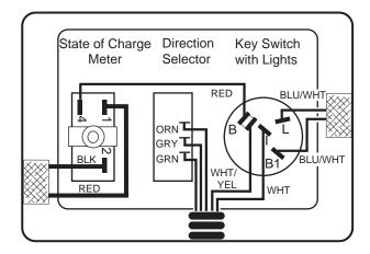
Fig. 3 Direction Selector Switch Connections
