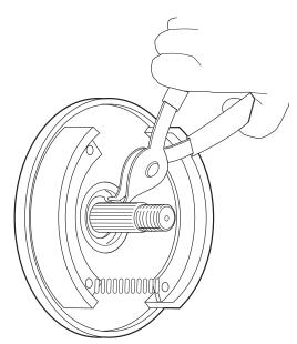
Fig. 2 Removing/Installing Outer Snap Ring
