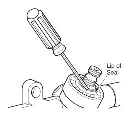
Fig. 15 Pinion Seal Replacement
