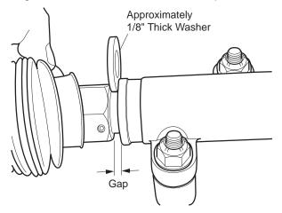
Fig. 19 Checking Gap
