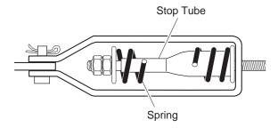
Fig. 3 Compensator Assembly
