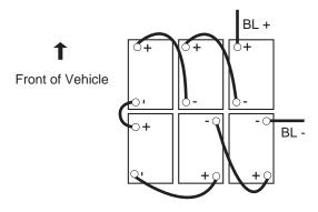
Fig. 5 Battery Connections
