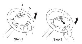
Fig. 20 Clipboard Removal
