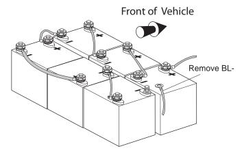
Fig. 1 Disconnect Battery Cable
