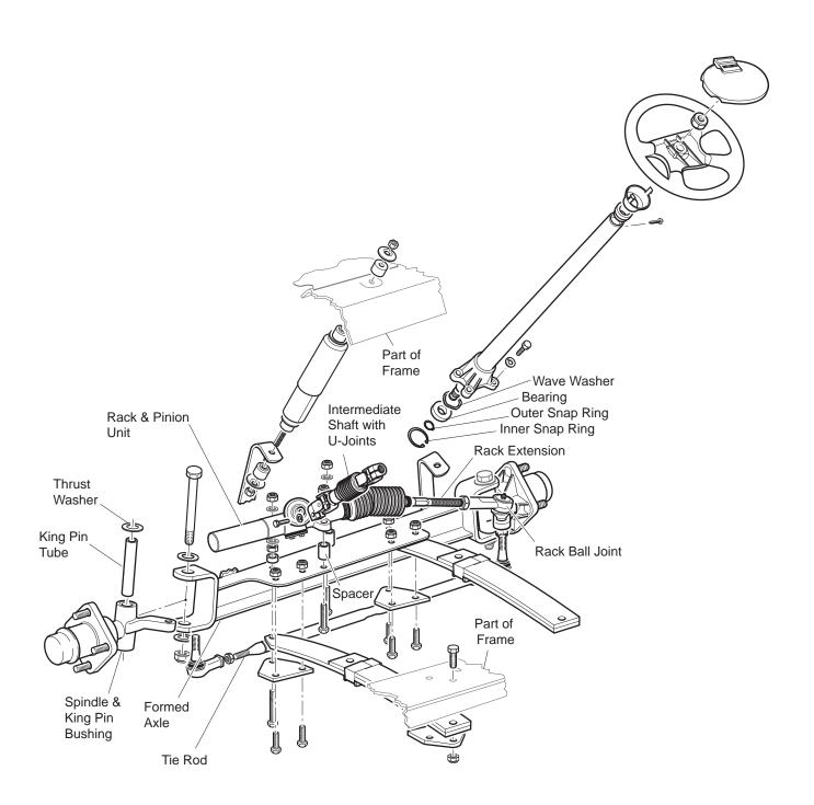
Fig. 1 Axle Mounted Steering and Front Suspension
