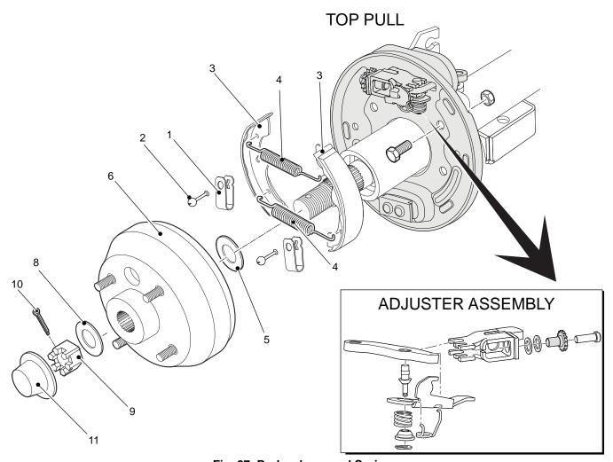
Fig. 27 Brake shoes and Springs
