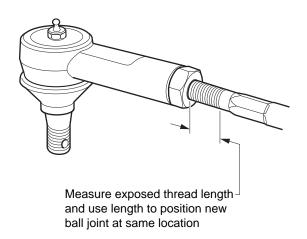
Fig. 12 Rack Ball Joint Installation
