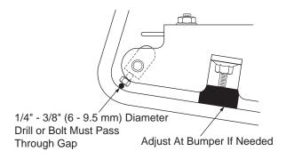
Fig. 7 Brake Pedal Bumper Inspection
