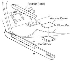
Fig. 2 Access to Pedal Box
