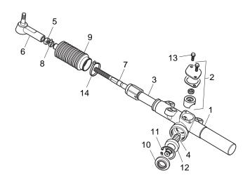
Fig. 17 Rack and Pinion Unit Disassembly
