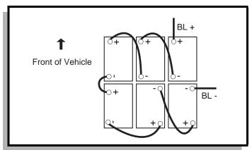
Fig. 1 Battery Connections
