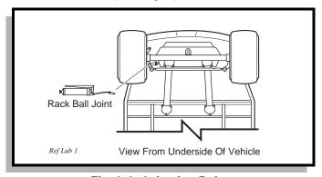
Fig. 2 Lubrication Point
