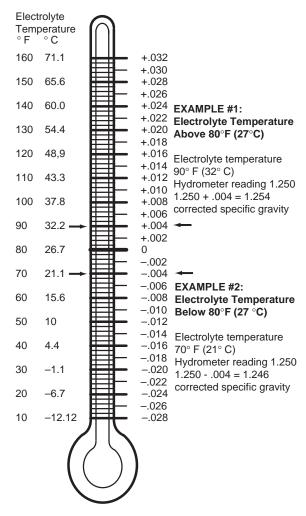
Fig. 8 Hydrometer Temperature Correction
