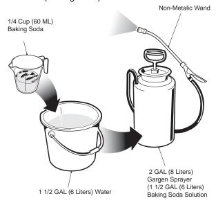
Fig. 4 Preparing Acid Neutralizing Solution
