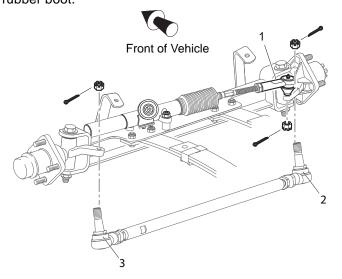
Fig. 2 Lubrication Points
