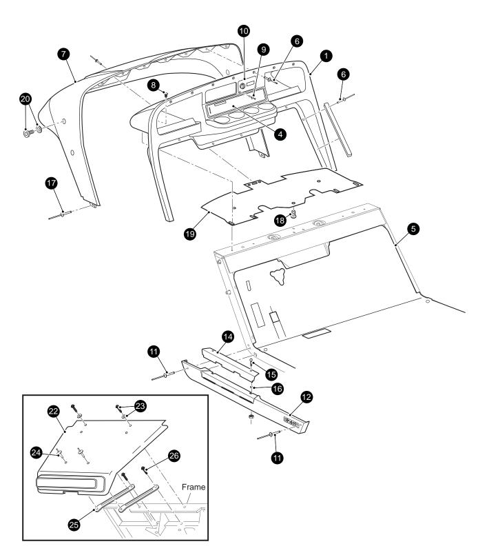
Fig. 2 Body Components (Front)
