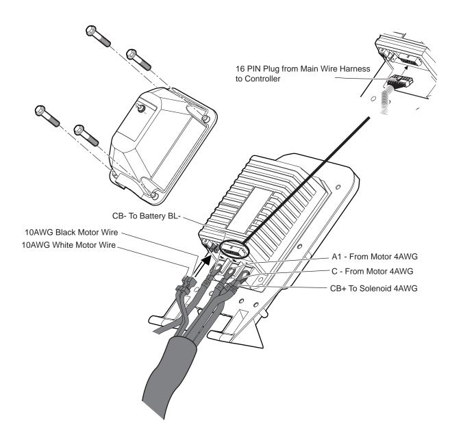
Fig. 8 Controller Connectors and Connections
