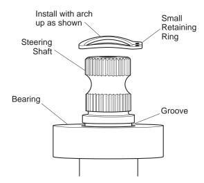
Fig. 23 Small Retaining Ring Orientation
