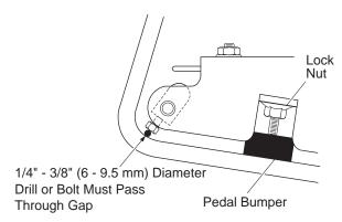
Fig. 30 Pedal Bumper Adjustment
