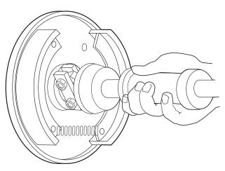
Fig. 6 Removing Seal
