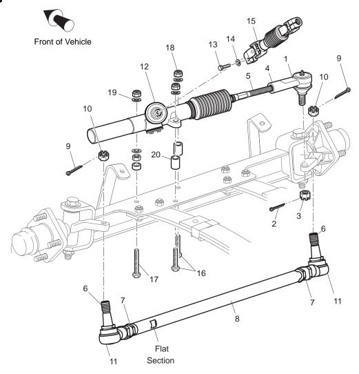
Fig. 11 Steering Components
