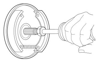
Fig. 3 Removing/Installing Axle Shaft
