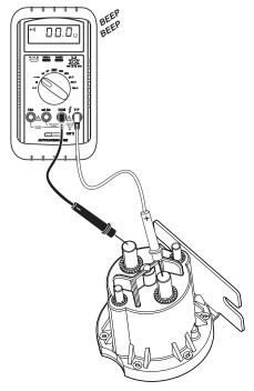
Fig. 6 Continuity Check of Solenoid
