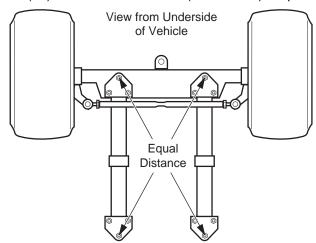
Fig. 7 Front Axle Alignment
