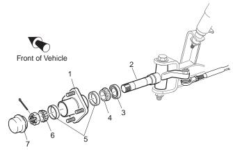
Fig. 10 Wheel Bearing Replacement
