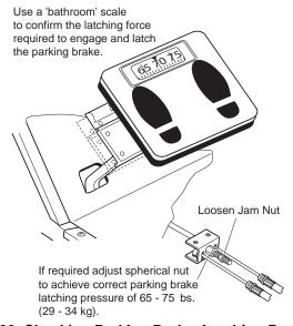
Fig. 20 Checking Parking Brake Latching Pressure
