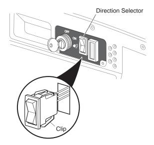
Fig. 2 Direction Selection Switch Replacement
