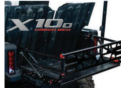
The Seizmik Bed Extender for the Honda Pioneer 1000-5 and 700-4 increases the amount of usable storage space in the vehicle. The additional area allows extra storage and hauling capacity, even when the rear seats are in use.
