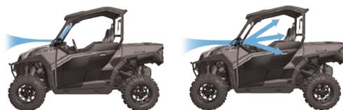
When placed in 'defog' mode, the vent directs outside air onto the inside surface of the windshield to help prevent fogging.
