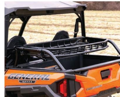
Secure and carry cargo above the dump bed of your General. The basket measures 42" x 20" and sits 4.5" above the dump bed edge. Side rails are 9" tall and there is a 100 lb weight limit.
