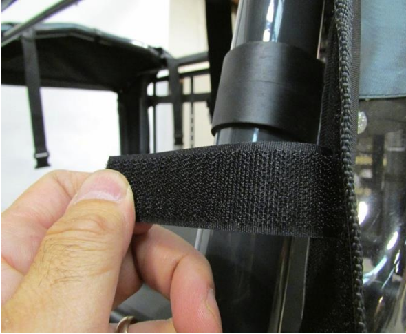
2. Securely fasten all Velcro straps around roll cage
