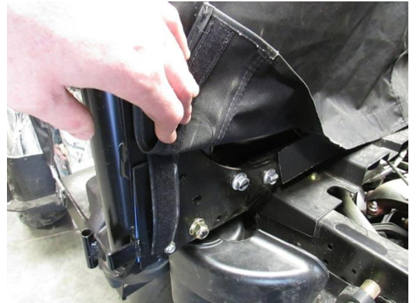
4. Note Velcro on inside edges of side panels along roll cage, & on lower body. Peel off self adhesive backing & stick to roll cage & body.
